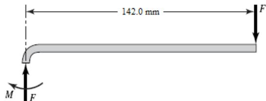
$M = 142F \text{ N}\cdot\text{mm}$ ,  $A = 4(20) = 80 \text{ mm}^2$ ,  $h = 4 \text{ mm}$ ,  $r_i = 4 \text{ mm}$ ,  $r_o = r_i + h = 8 \text{ mm}$ ,
